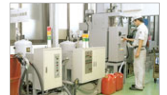
Wasted production oil is 97% recycled after being purified via special filtration equipment.
