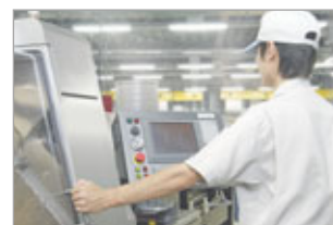
NC lathe process – Even during computer-controlled production, the automated process is monitored by a skilled operator to ensure the highest quality of micro precision production.
