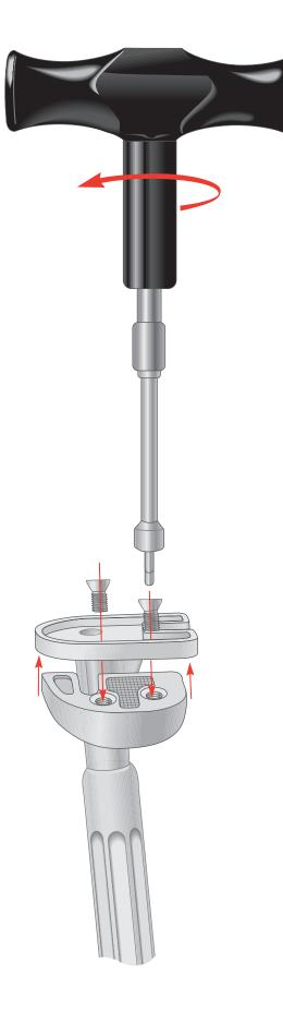
Where wedge augmentation is indicated, the appropriate polyethylene plugs are removed from the Modular Plus tibial tray with the plug puller.
