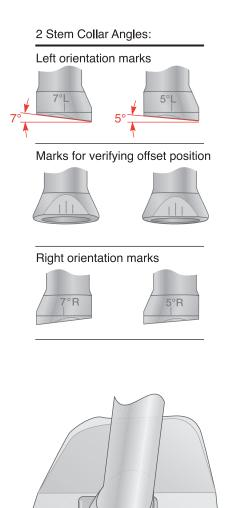
Orientation system to verify angulation and left/right orientation.
