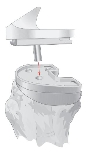
The anterior and posterior margins are simultaneously deflected past the lip of the tray and into position by tapping with a poly tibial component impactor. Seating is confirmed by circumferential inspection.
